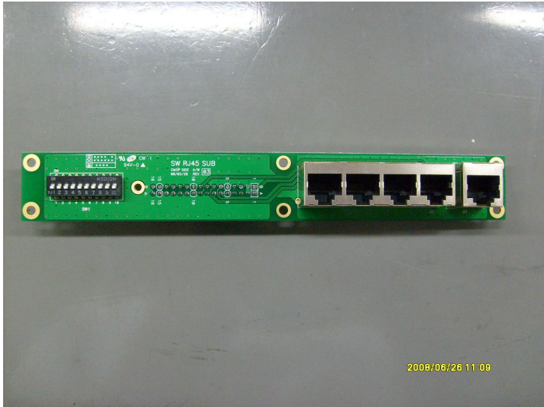
&lt;Photograph 12: Internal - (RJ45) FRONT view&gt;
