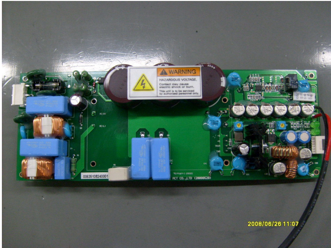
<Photograph 6: Internal - (AC-DC converter) FRONT view>
