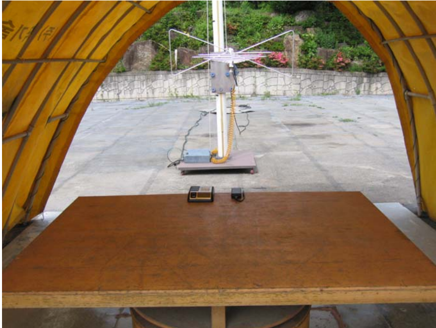
Photograph 1 : Setup for radiated Emissions
