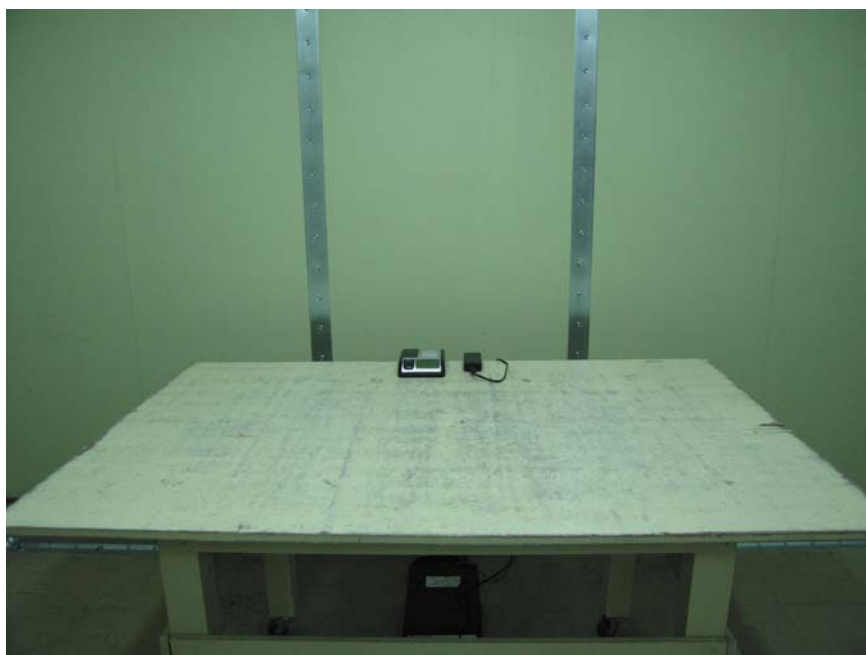
Photograph 2 : Setup for Conducted Emissions
