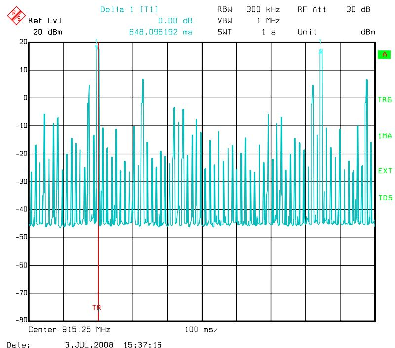
That gives a maximum of 1 transmissions in a period of 100 ms so the duel time correction factor for spurious measurement is  $20\log(1x6.53/100) = -23.70 \text{ dB}$ .
