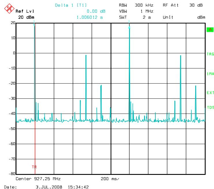
That gives a maximum of 1 transmissions in a period of 100 ms so the duel time correction factor for spurious measurement is  $20\log(1x7.02/100) = -23.07 \text{ dB}$ .
