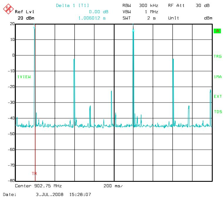
That gives a maximum of 1 transmissions in a period of 100 ms so the duel time correction factor for spurious measurement is  $20\log(1x6.97/100) = -23.14 \text{ dB}$ . But the worst case of a real communication has been measured by the manufacturer to be 200 ms. That gives a correction factor of **0 dB**.
