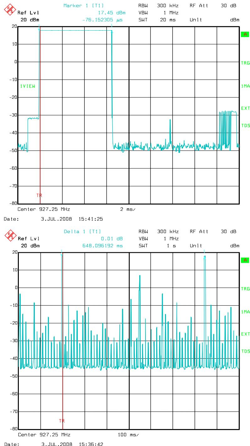
That gives a maximum of 1 transmissions in a period of 100 ms so the duel time correction factor for spurious measurement is  $20\log(1 \times 6.55/100) = -23.74 \text{ dB}$ .
