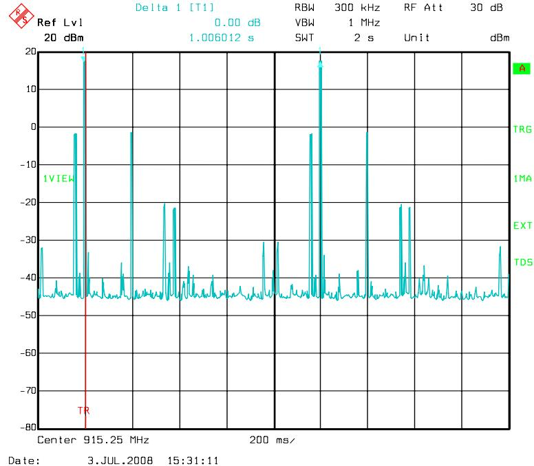
That gives a maximum of 1 transmissions in a period of 100 ms so the duel time correction factor for spurious measurement is  $20\log(1x7.01/100) = -23.09 \text{ dB}$ .
