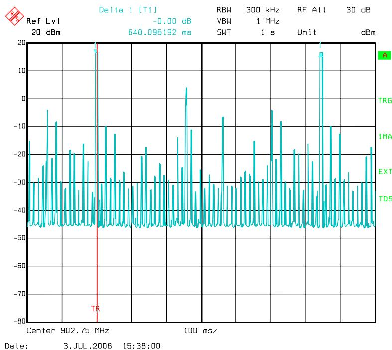
That gives a maximum of 1 transmissions in a period of 100 ms so the duel time correction factor for spurious measurement is  $20\log(1 \times 6.53/100) = -23.70 \text{ dB}$ . But the worst case of a real communication has been measured by the manufacturer to be 18ms. That gives a correction factor of **-14.9 dB**.
