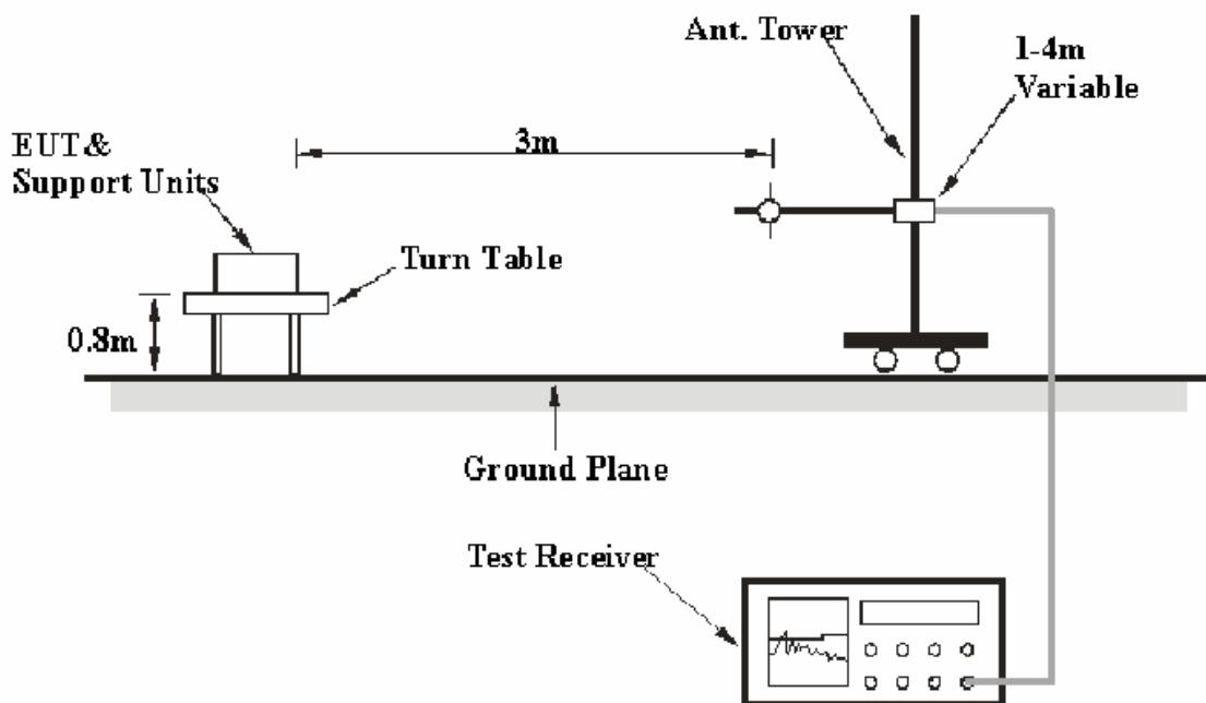
The radiated emission tests were performed in the 3 meters chamber B test site, using the setup accordance with the ANSI C63.4-2003. The specification used was the FCC 15.109, FCC 15.209 and FCC 15.247 limits.
