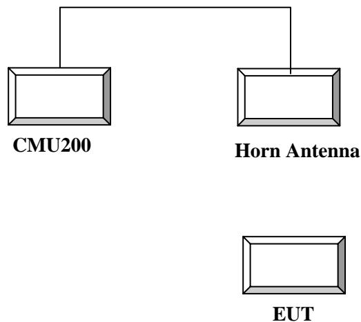
**Block Diagram of Test Setup****Charging mode:**
