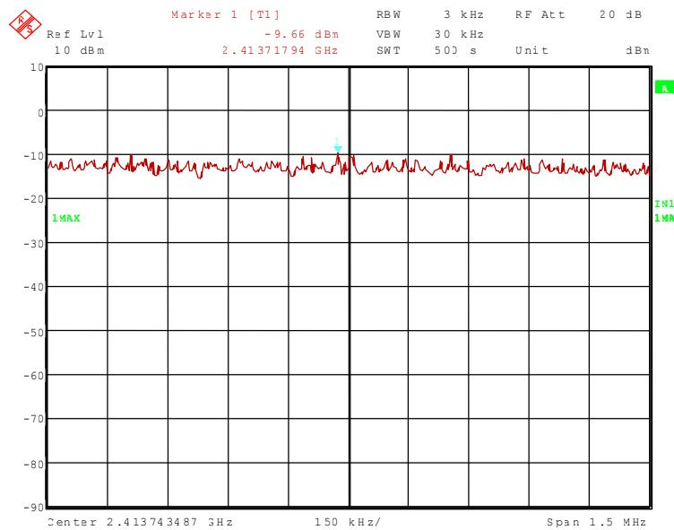
80804\_91.wmf (power spectral density (transmit on channel 6)):
