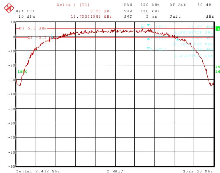
80804\_87.wmf: (6 dB bandwidth at the middle of the assigned frequency band):
