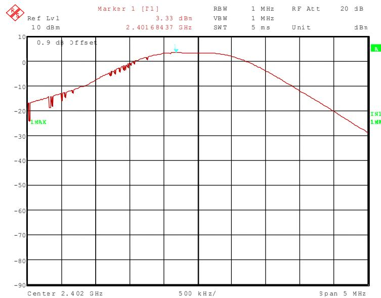
80804\_77.wmf (maximum peak output power at the middle of the assigned frequency band):
