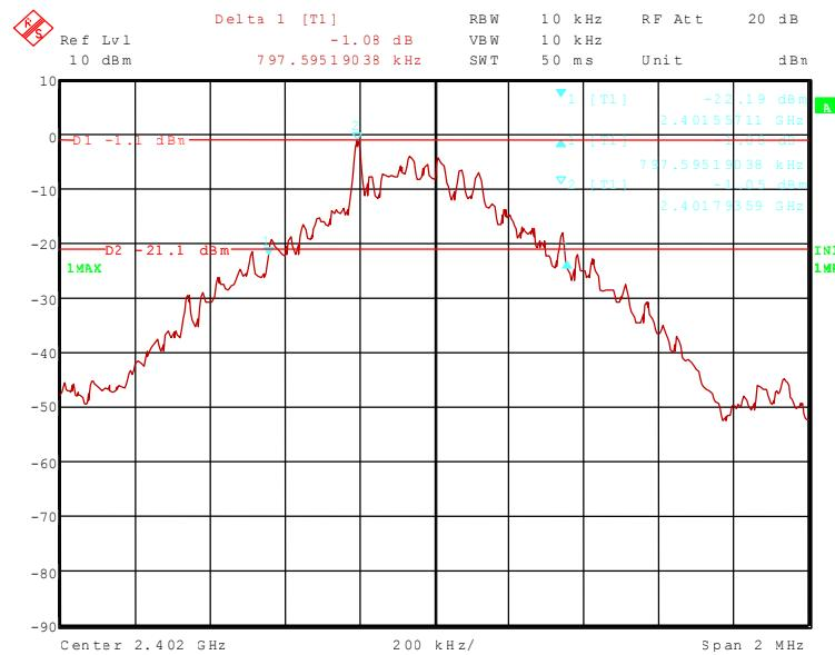
80804\_74.wmf: (20 dB bandwidth at the middle of the assigned frequency band):
