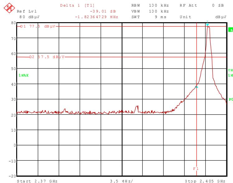
80804\_70.wmf (radiated band-edge compliance, lower band edge, hopping on):
