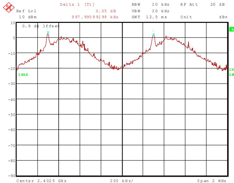
80804\_80.wmf: (channel separation at the middle of the assigned frequency band):
