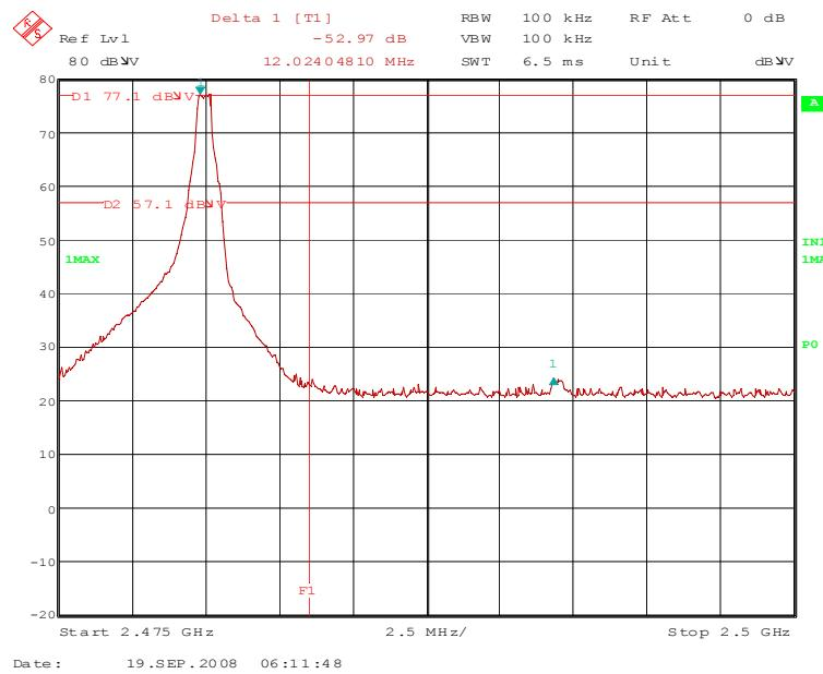
80804\_71.wmf (radiated band-edge compliance, upper band edge, hopping on):
