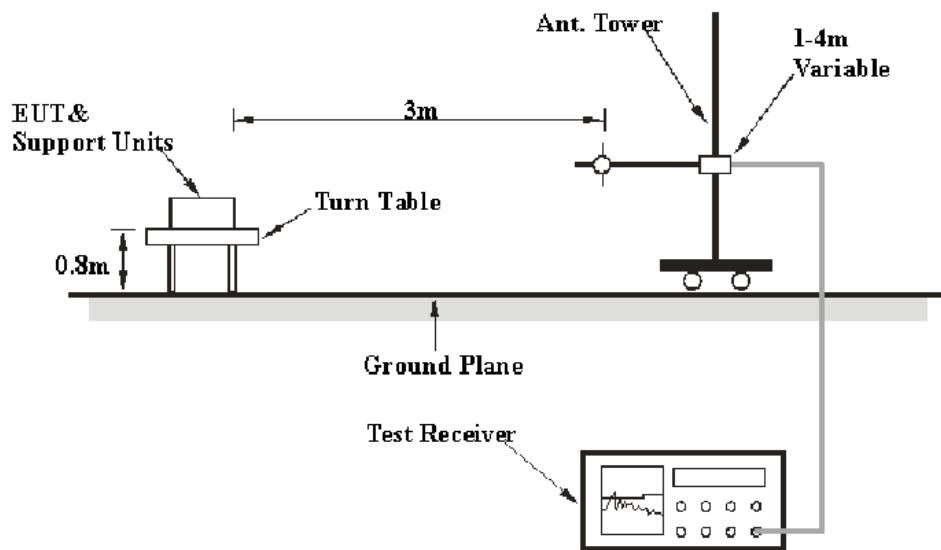
The radiated emission tests were performed in the 3 meters test site, using the setup accordance with the ANSI C63.17 2013. The specification used was the FCC 15§ 15.319(g).
