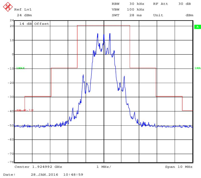
**High Channel (Unwanted Emission inside the Sub-band)**
