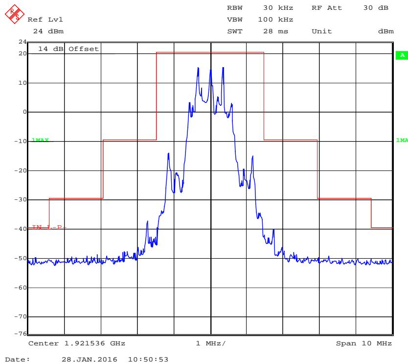
**Middle Channel (Unwanted Emission inside the Sub-band)**
