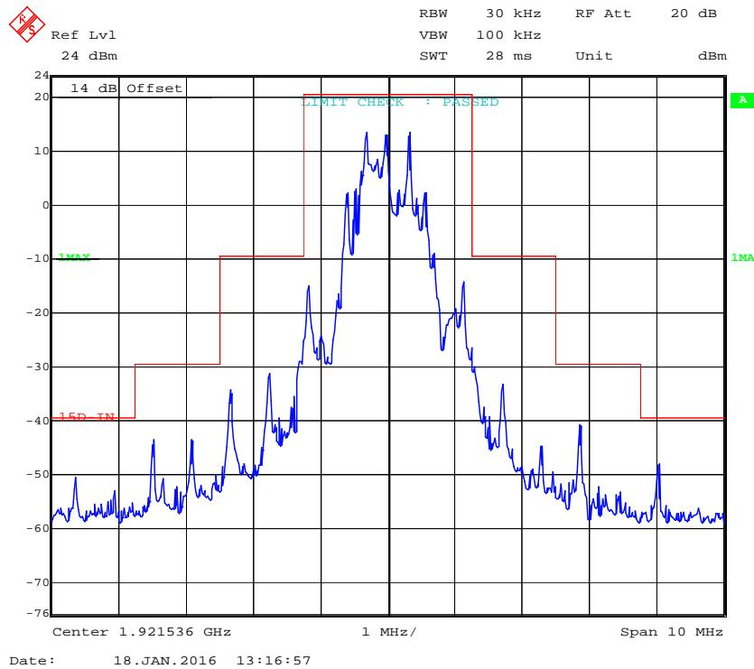
**Middle Channel (Unwanted Emission inside the Sub-band)**
