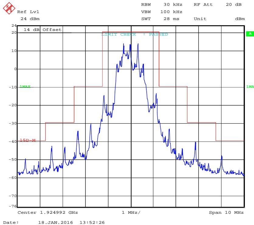
**High Channel (Unwanted Emission inside the Sub-band)**
