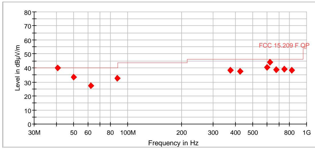
The results of the standard subsequent measurement on the open area test site are indicated in the table below. The limits as well as the measured results (levels) refer to the above mentioned standard while taking account of the specified requirements for a 3 m measuring distance.
