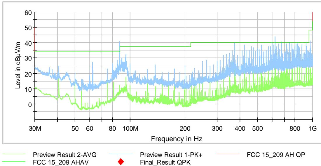
Remark: As pre-test have shown, reading a 13.56 MHz TAG causes higher emissions above 30 MHz. Therefore the tests above 30 MHz were carried out with this TAG
