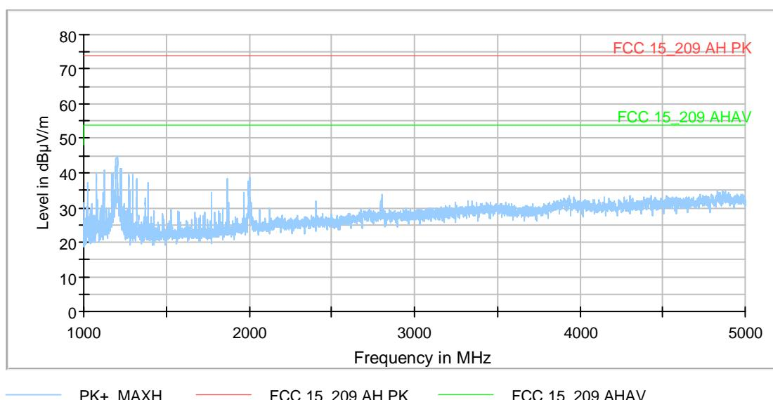
Remark: As pretest has shown, reading a 13.56 MHz TAG causes higher emissions above 30 MHz. Therefore the tests above 30 MHz were carried out with this TAG
