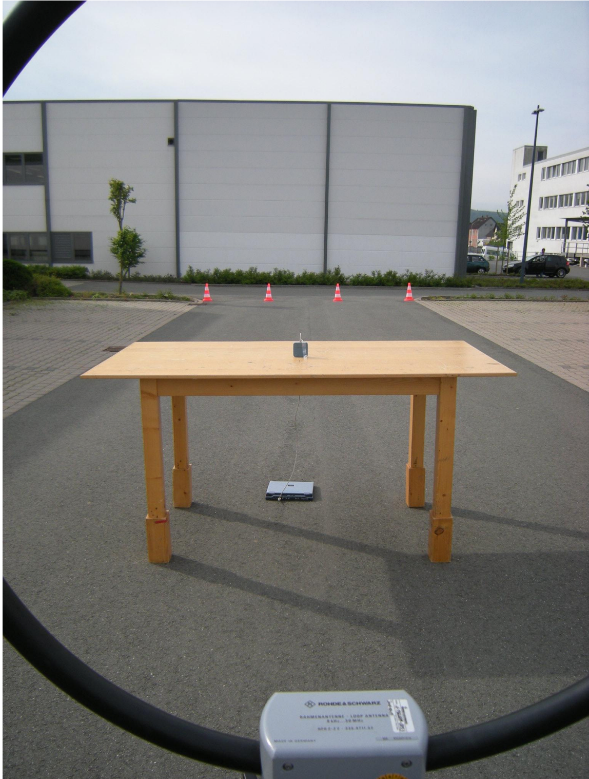
91053emi_fcc7.jpg: Test set-up outdoor test site
