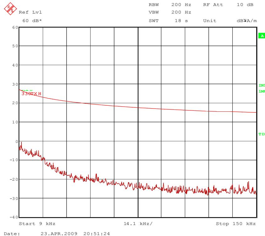
91053tx1.wmf: Spurious emissions from 9 kHz to 150 kHz
