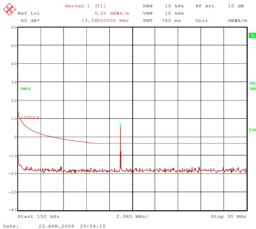
**91050tx2.wmf: Spurious emissions from 150 kHz to 30 MHz**
