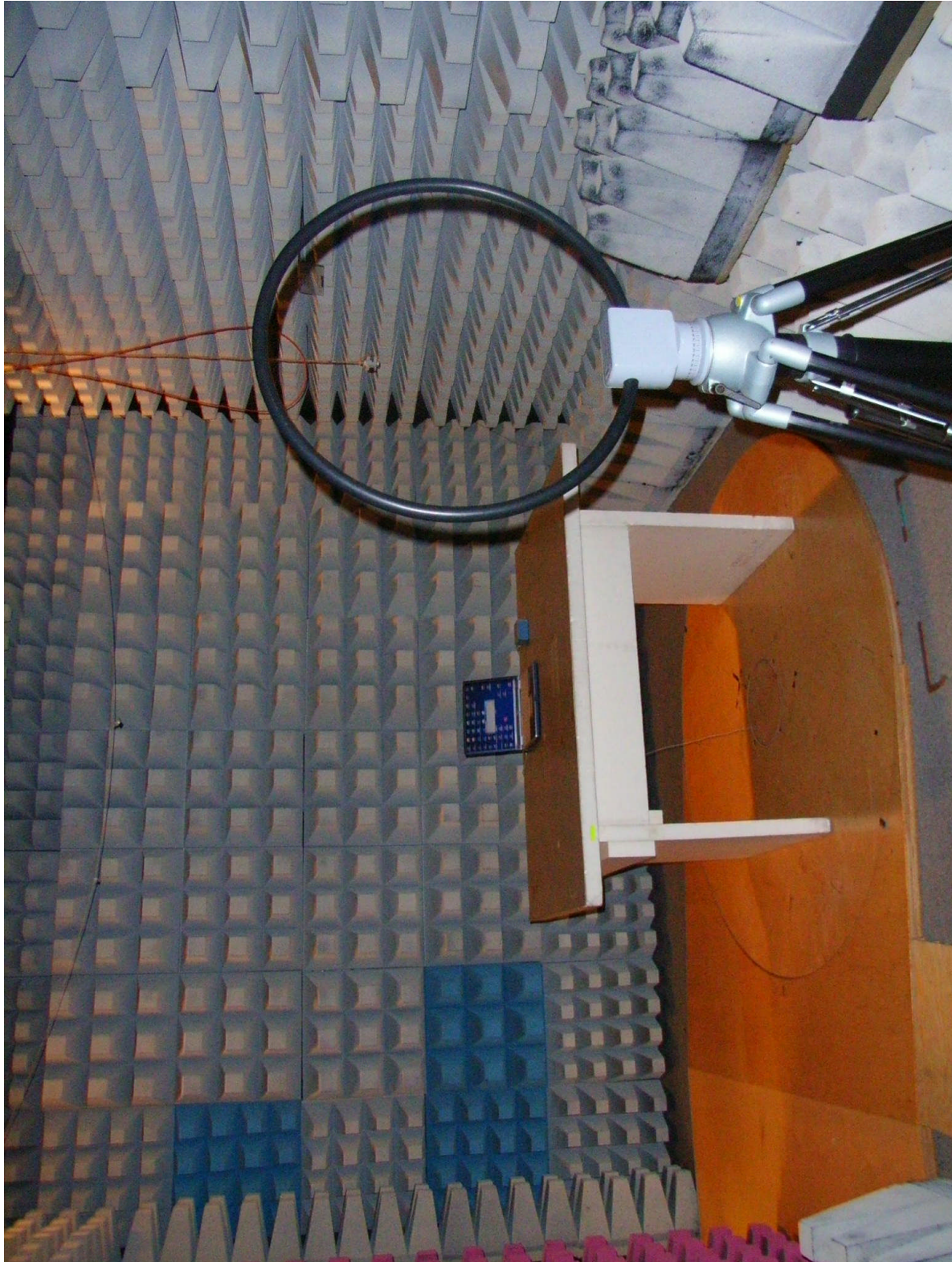
82825emi5.jpg Test set-up fully anechoic chamber (H-Field)
