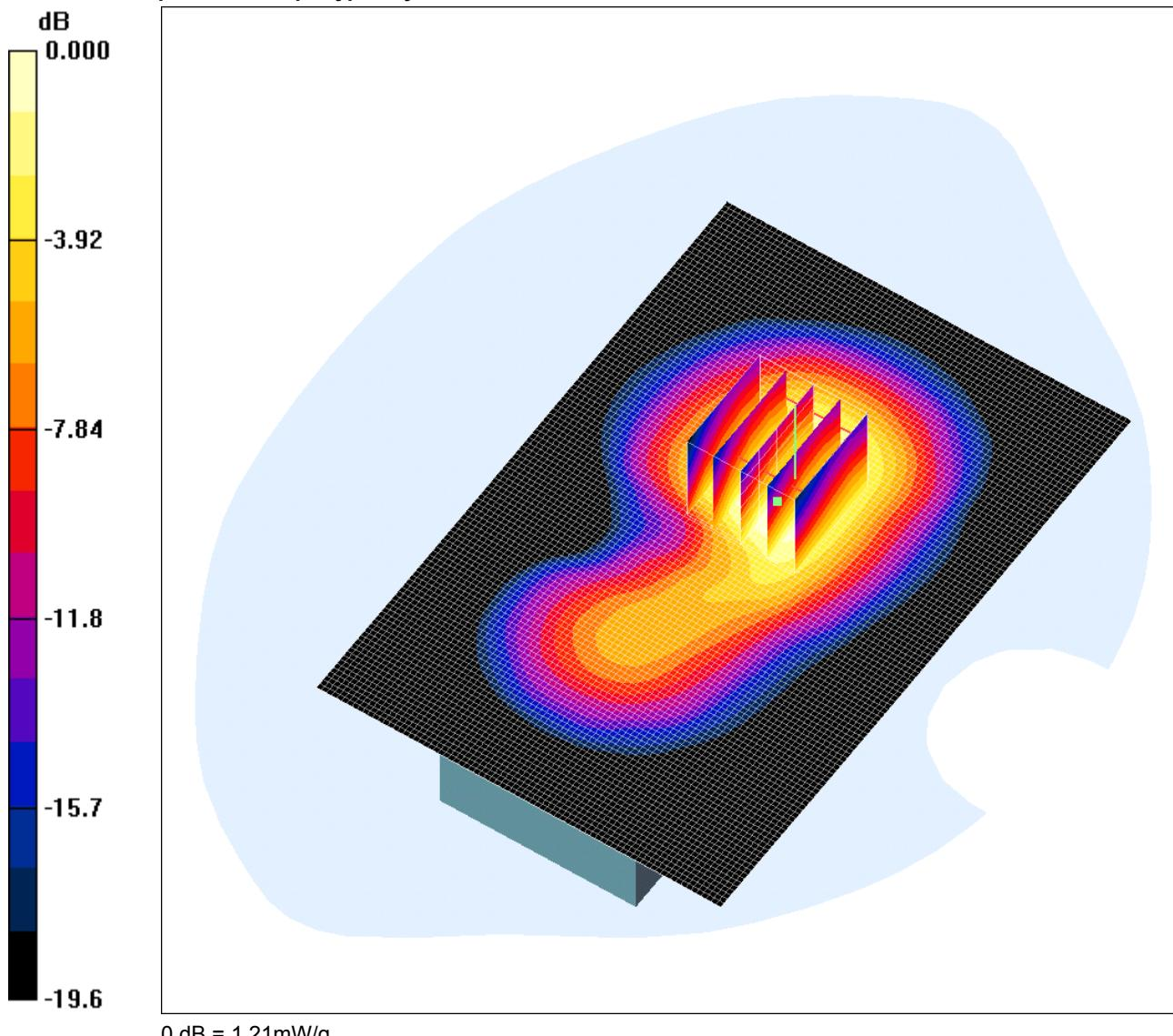
Communication System: GPRS 1900; Frequency: 1879.8 MHz; Duty Cycle: 1:4
