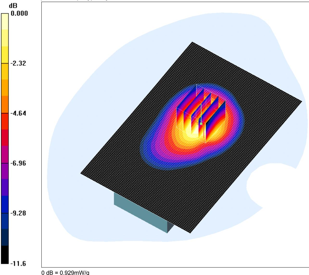
Communication System: GPRS 850 MHz; Frequency: 836.4 MHz; Duty Cycle: 1:4
