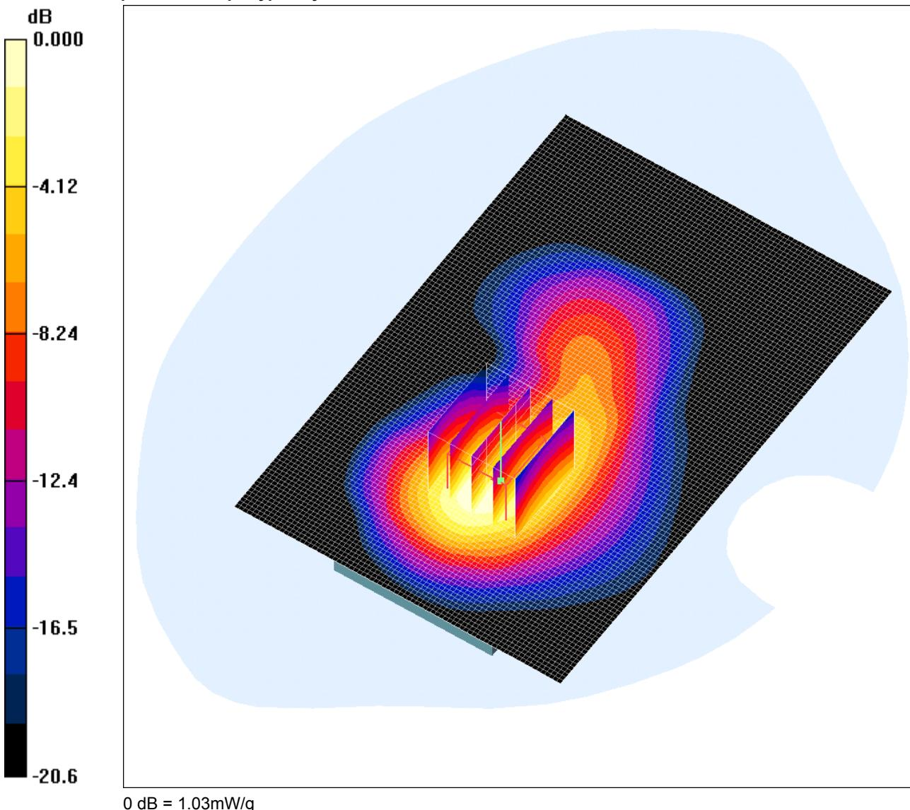
Communication System: GPRS 1900; Frequency: 1850.2 MHz; Duty Cycle: 1:4
