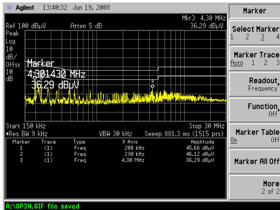
**Plot of Conducted Emissions Test Data***Conducted Disturbance**EUT: Clip Bluetooth Mp3**M/N: SPB01**Operating Condition: Downloading**Test Specification: L**Comment: AC120V/60Hz; Connected to PC, USB 5V*
