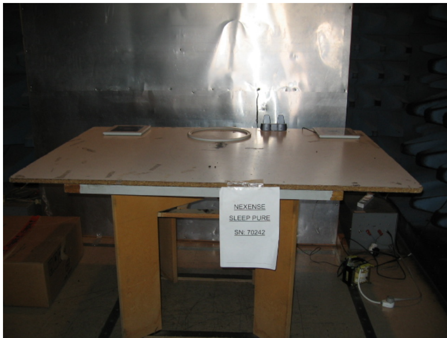
Figure 2. Conducted Emission Test
