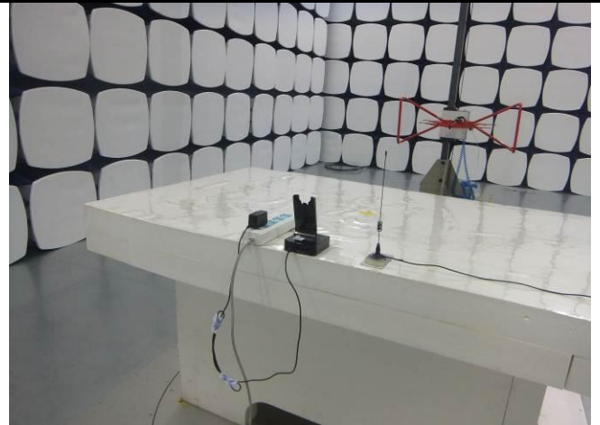
Radiated Spurious Emissions Test Setup Below 1GHz
