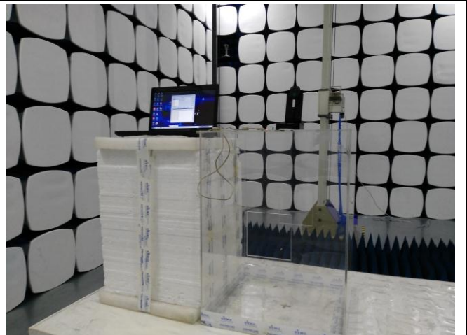
Radiated Spurious Emissions Test Setup Above 1GHz
