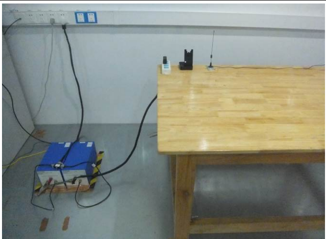
Radiated Spurious Emissions Test Setup Above 1GHz
