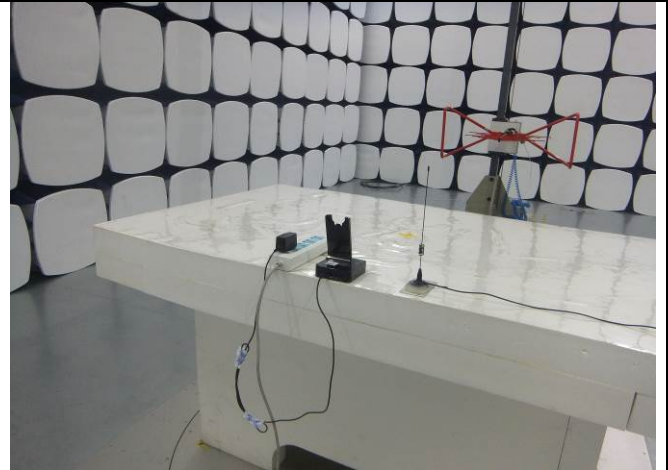
Radiated Spurious Emissions Test Setup Below 1GHz
