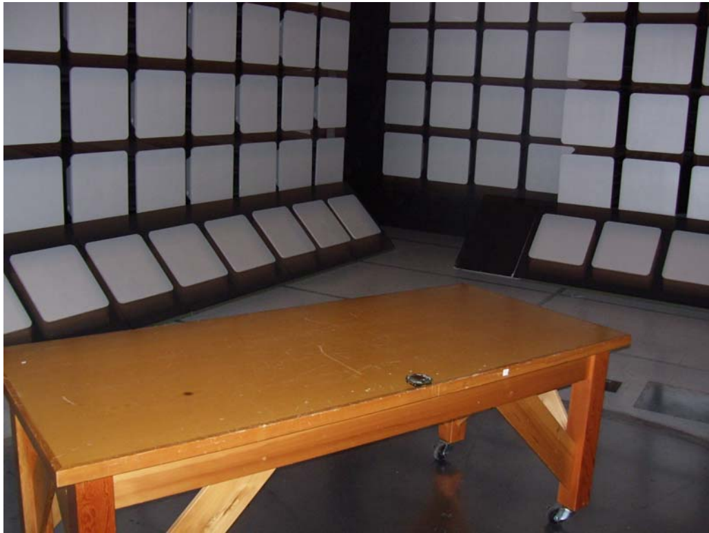
Figure 13 - Radiated Emissions Test Setup
