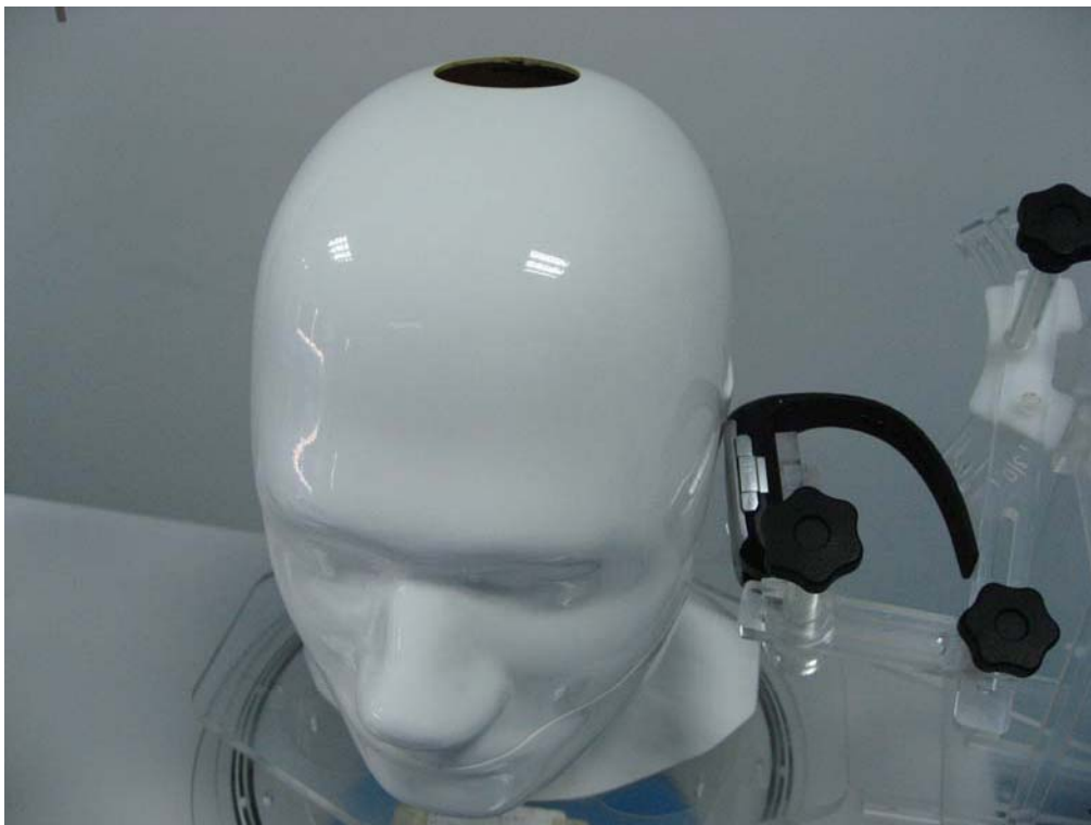
Fig.4 EUT Left Head Tilt15 Position
