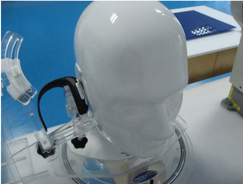
Fig.5 EUT Right Head Touch Cheek Position
