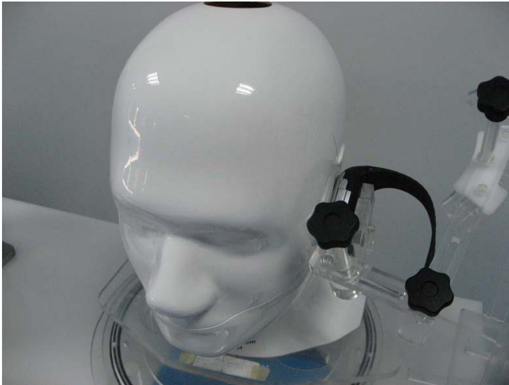
Fig.3 EUT Left Head Touch Cheek Position
