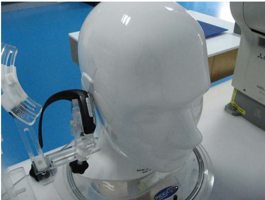
Fig.6 EUT Right Head Tilt15 Position
