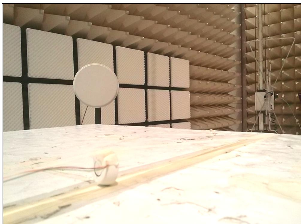
**C. Photo of Radiated Spurious Emission Test (Above 1 GHz)**
