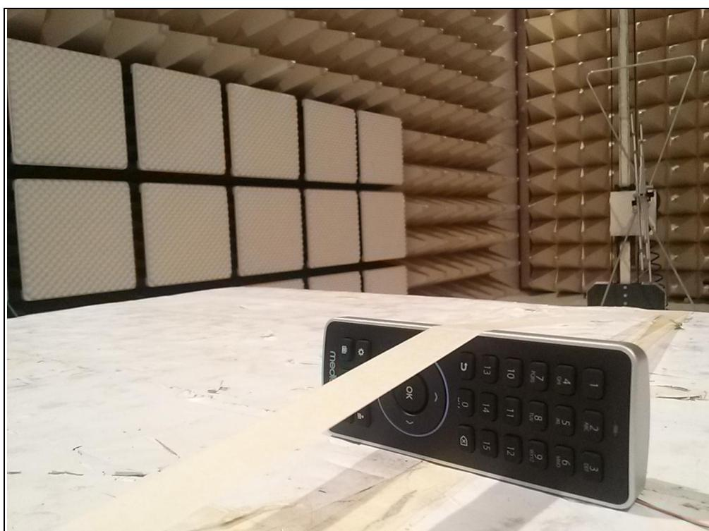
**C. Photo of Radiated Spurious Emission Test (Above 1 GHz)**
