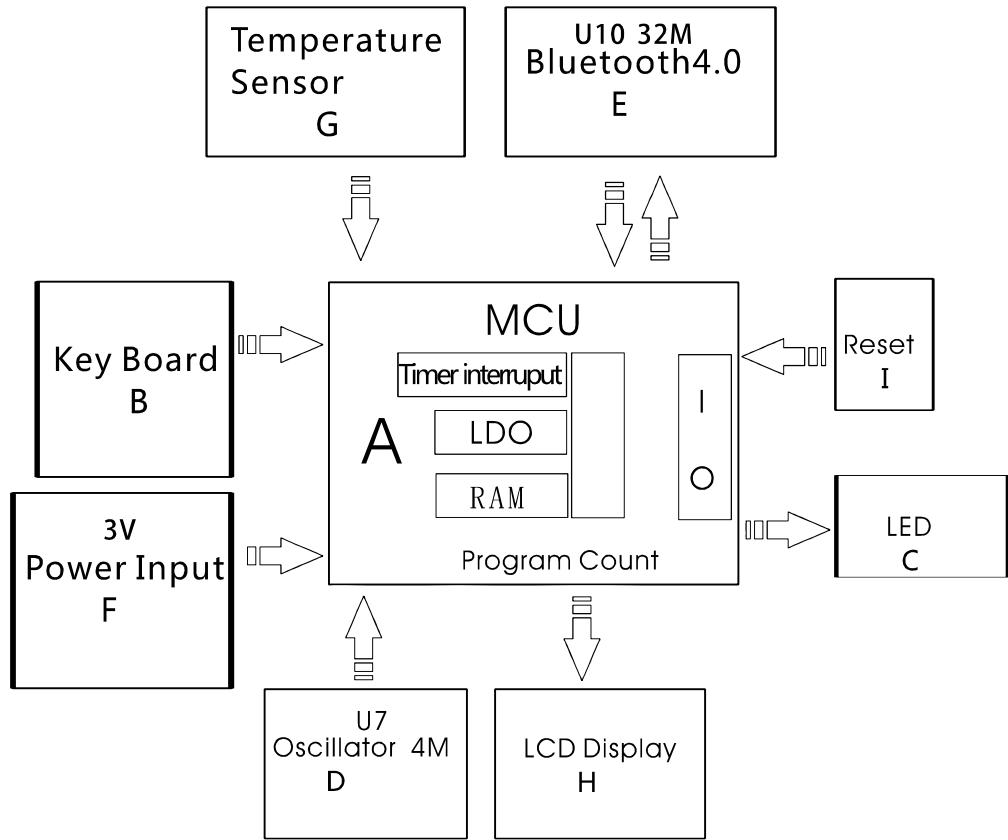
The device contains MCU temperature sensor, buttons, bluetooth modules and other devices.
