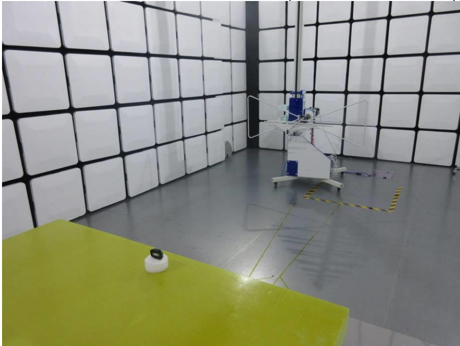
RADIATED RF MEASUREMENT SETUP (30MHz ~ 1 GHz - Y axis)
