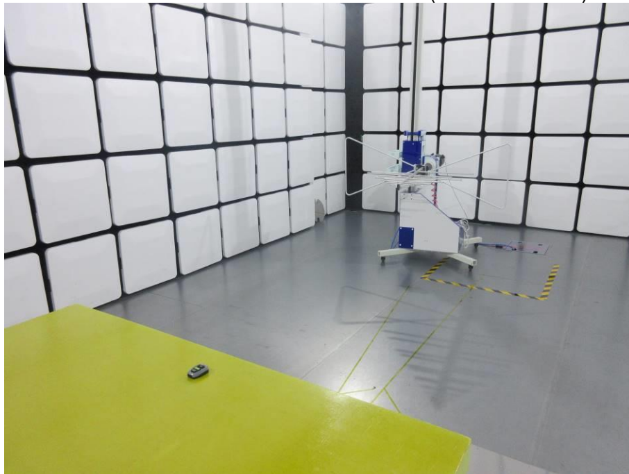
RADIATED RF MEASUREMENT SETUP (30MHz ~ 1 GHz)
