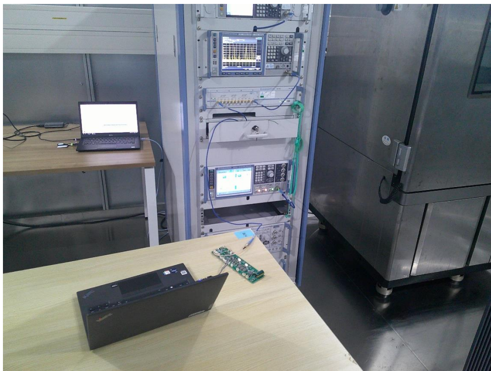
Photograph 1: Set-up photo for RF Conducted Test
