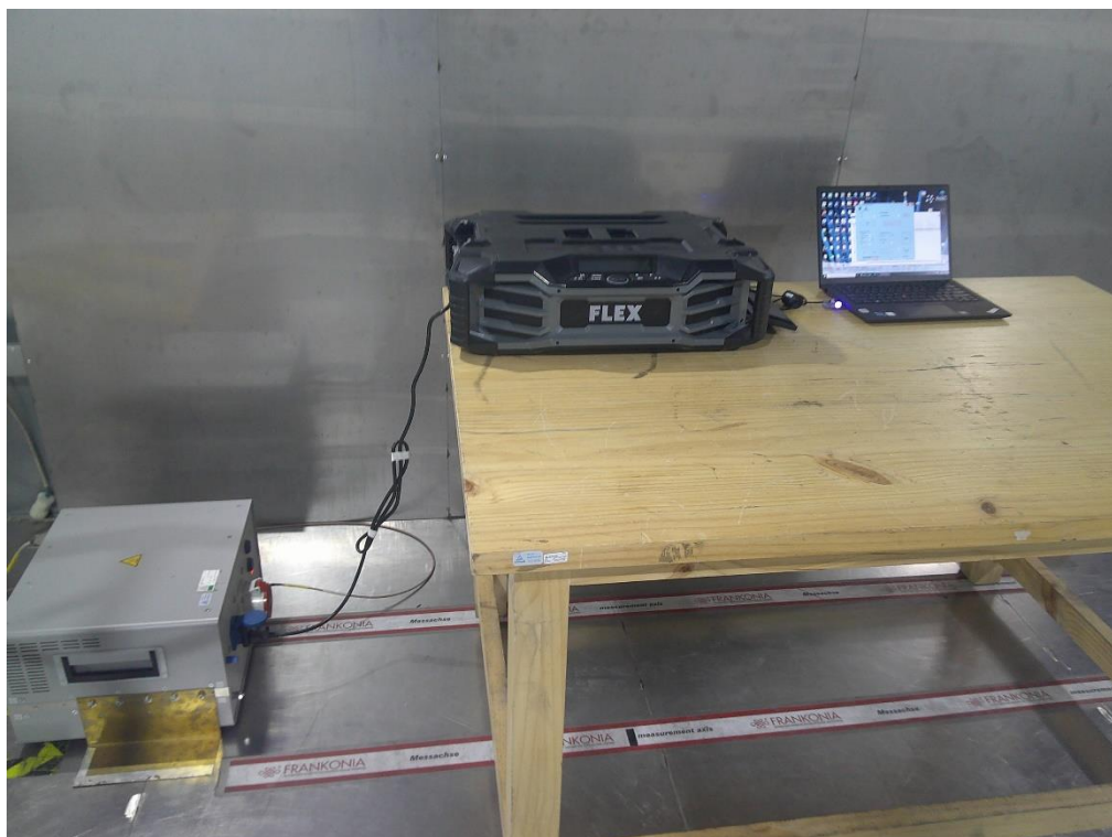
Photograph 2: Set-up photo for Conducted Emission
