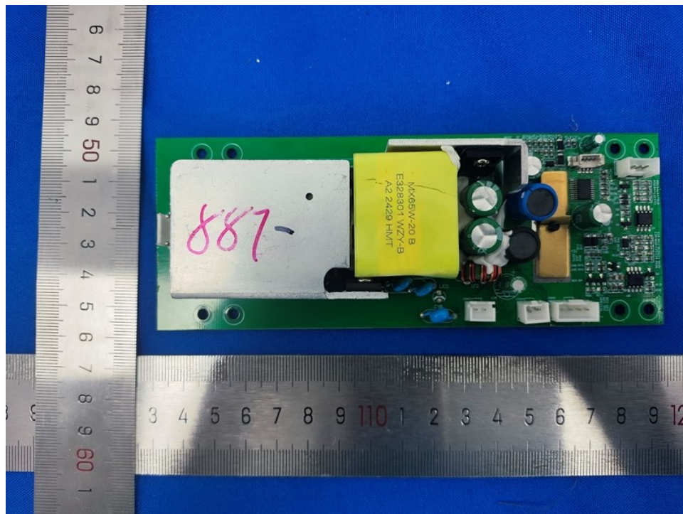
Bild / Picture 12: power board
