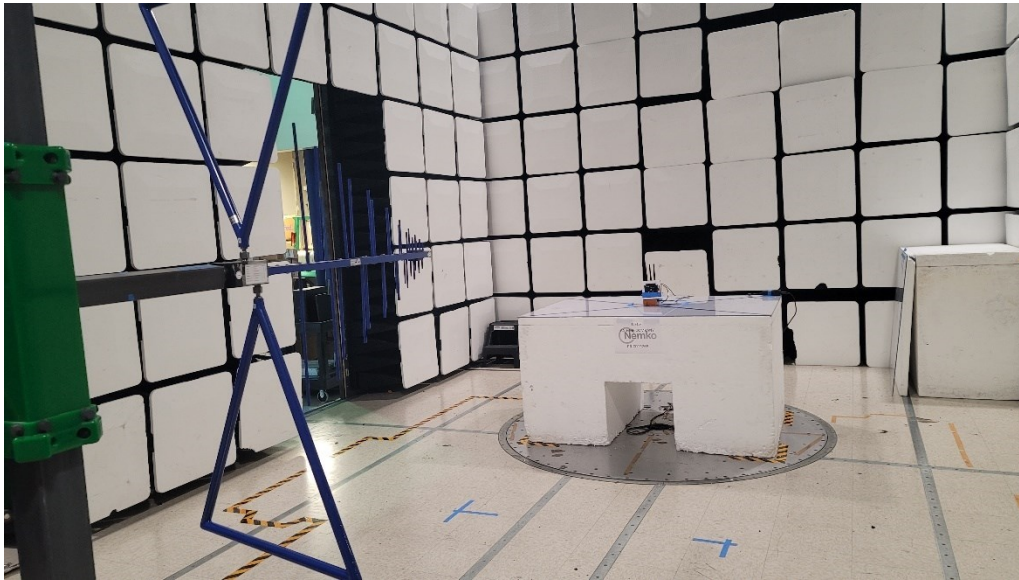
Figure 6 - Radiated emissions below 1 GHz (30 – 150 MHz), front view.
