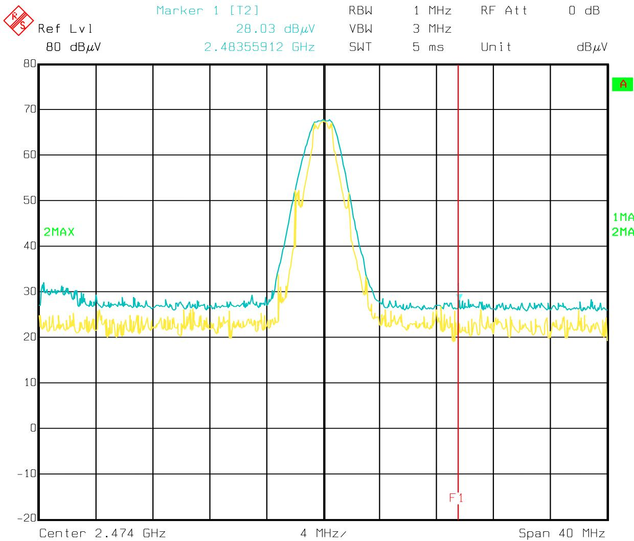
High Channel (2474MHz using 1MHz RBW/ 3MHz VBW)
