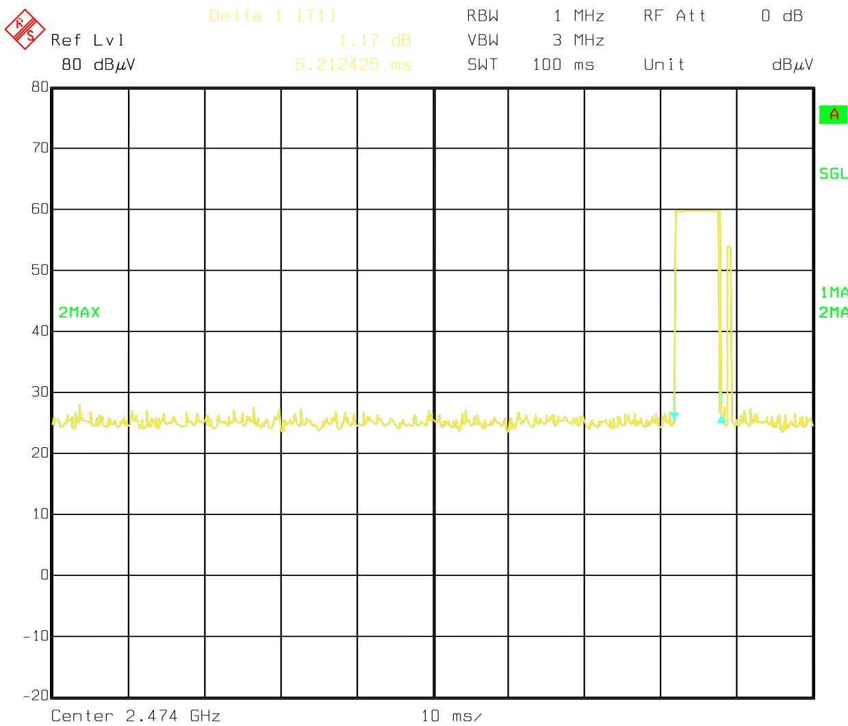
**Duty Cycle** $= 6.21 \text{ ms}/100\text{ms} = 6\%$ **Duty Cycle Factor** $= -20 \text{ dB}$  since duty cycle is < 10%
