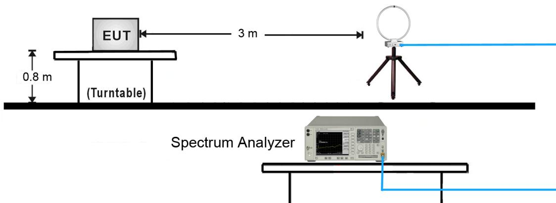
Below 1GHz Test Setup:
