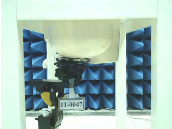
Figure 3. Left Head SAR Test Setup (Cheek)
