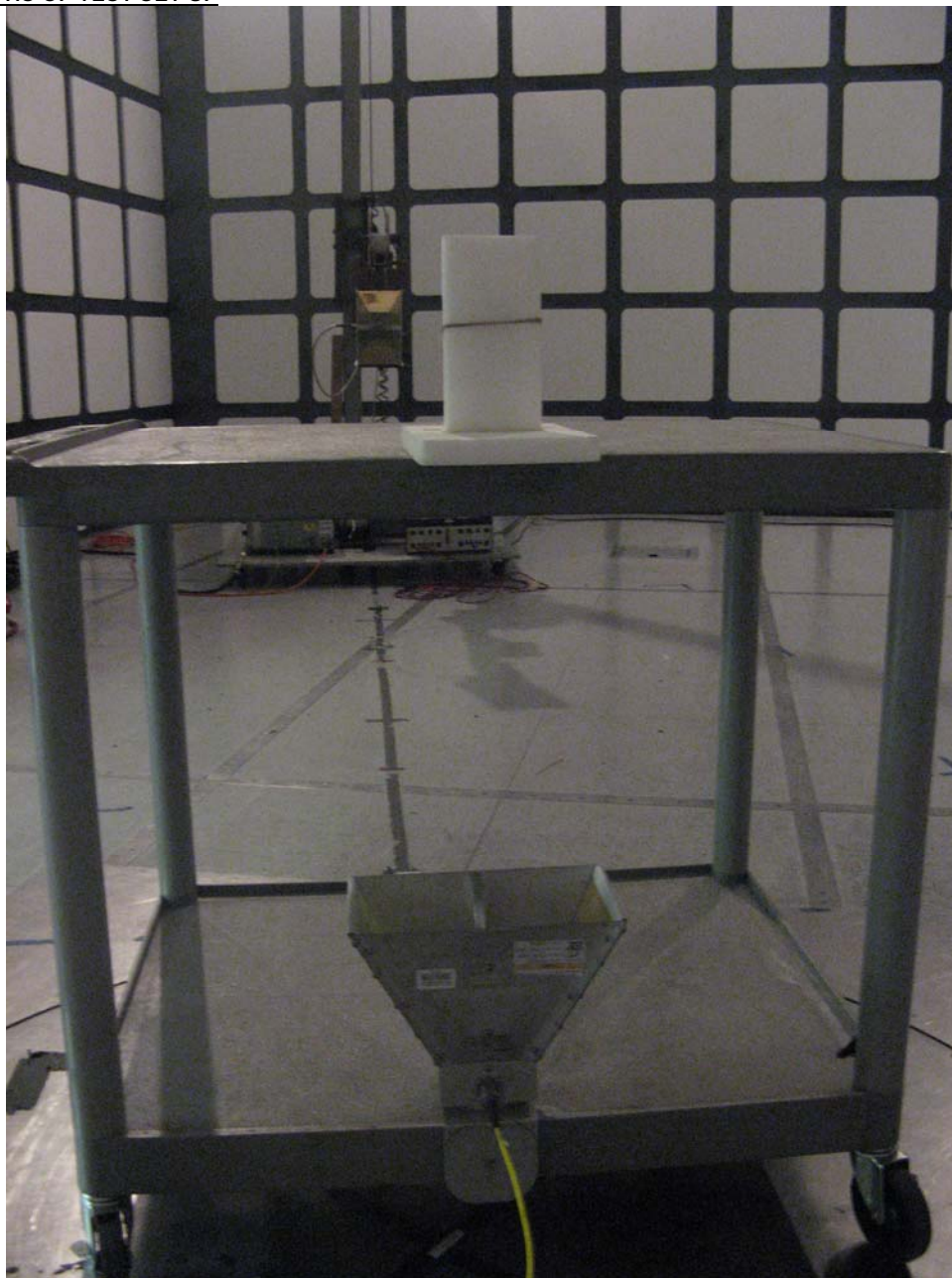
Radiated Emissions (Enclosure Port) Test Setup
