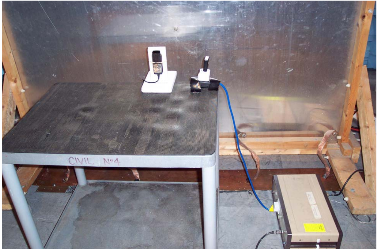
Conducted Emissions (AC Power Port) Test Setup
