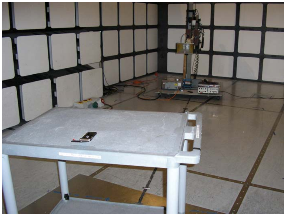
Radiated Emissions (Enclosure Port) Test Setup
