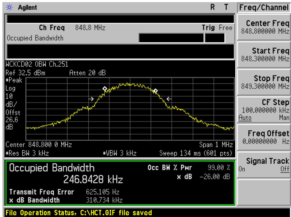
■ GSM850 EDGE (251 CH.) Occupied Bandwidth
