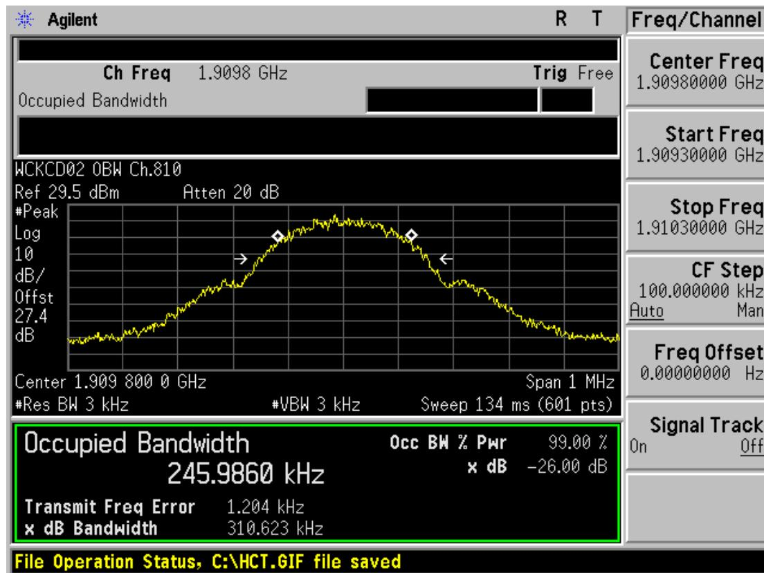
■ GSM1900 EDGE (512 CH.) Occupied Bandwidth
