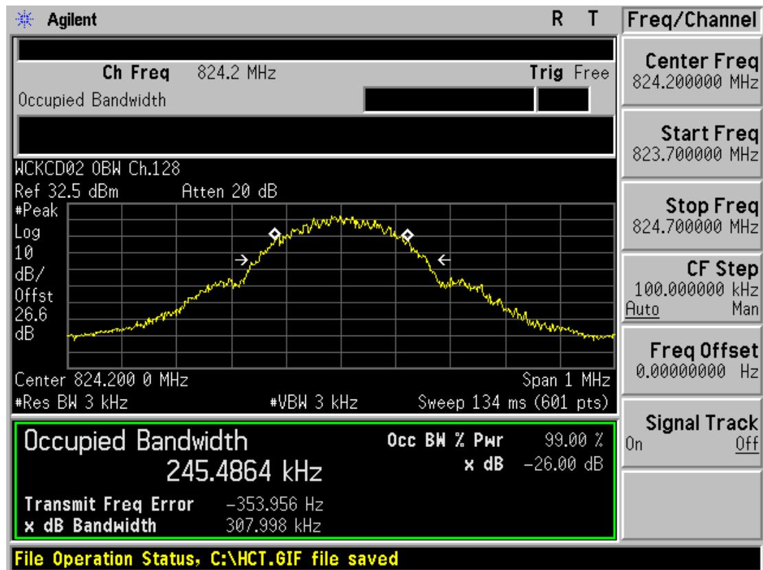
■ GSM850 MODE (190 CH.) Occupied Bandwidth
