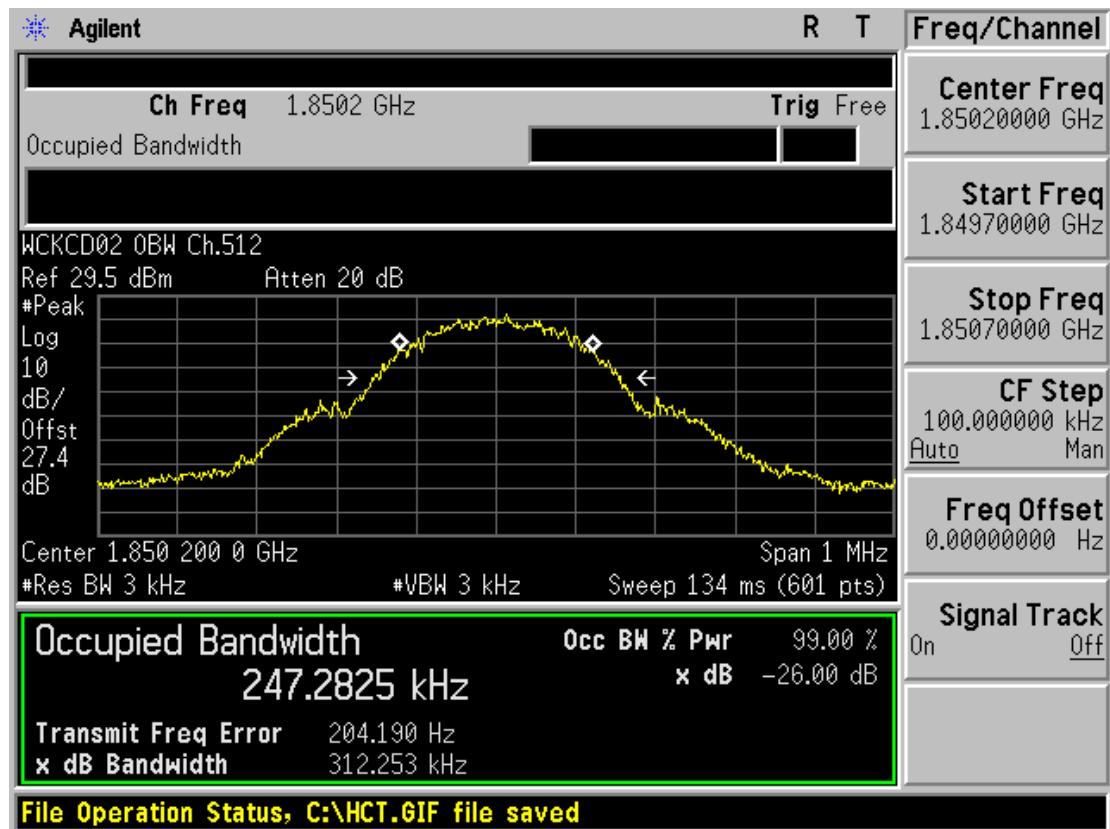
■ GSM1900 MODE (661 CH.) Occupied Bandwidth
