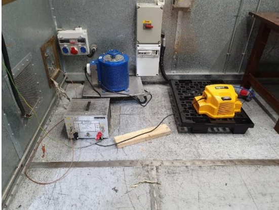
Photograph 8.1: Setup for conducted emission measurements, Transmitter BLE 2.44 GHz
