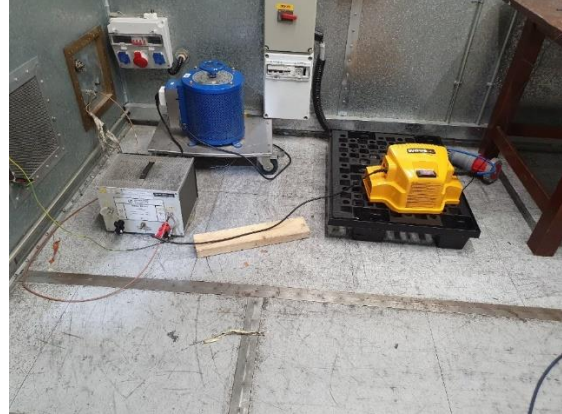
Photograph 8.1: Setup for conducted emission measurements, Transmitter BLE 2.44 GHz
