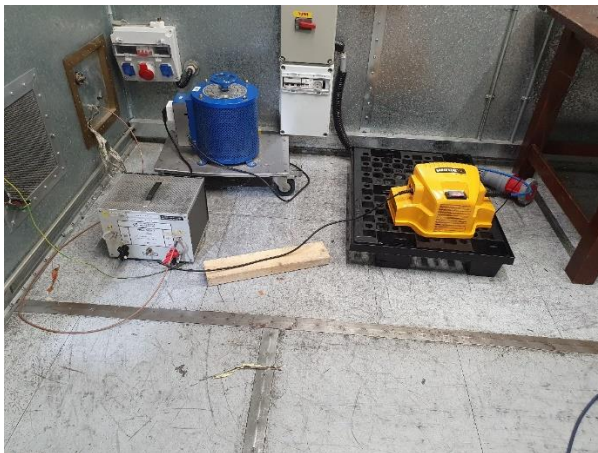
Photograph 8.2: Setup for conducted emission measurements, Receiver BLE 2.44GHz
