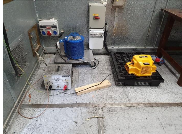
Photograph 8.2: Setup for conducted emission measurements, Receiver BLE 2.44GHz
