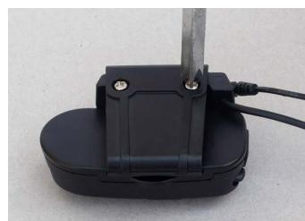
2. Slide the patch panel between the helmet hull and internal pad. (if the helmet hull is too thick, please use included extra thick clip. )
