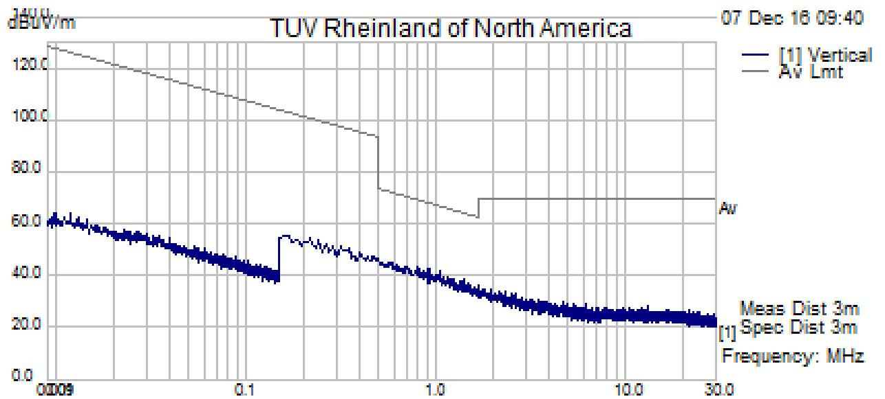
NeuroPace, RNS Neurostimulation, Model RNS 320, SN: 191391, TX mode at Z axis, loop 0 deg
