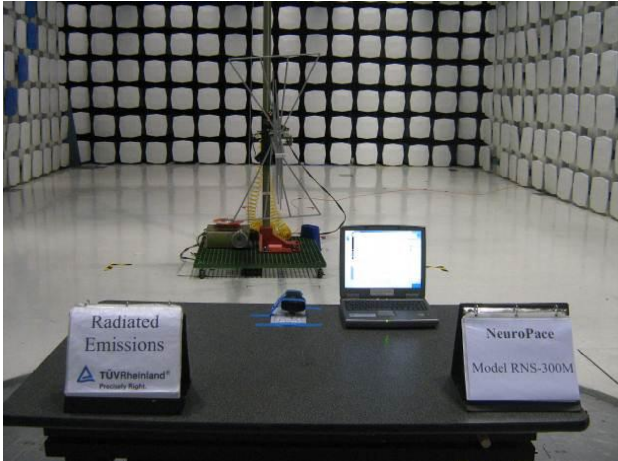
Figure 3: Test Setup for 30 MHz to 1000 MHz Radiated Emission (Front View)
