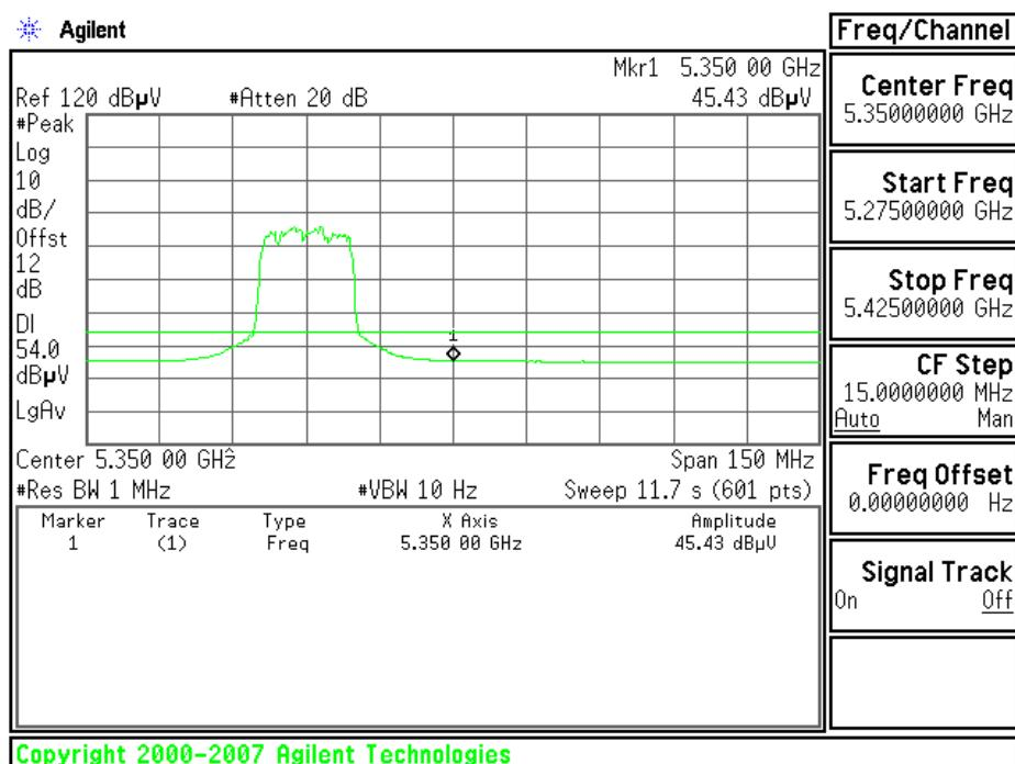
**Band Edges (draft 802.11n Standard-20 MHz Channel mode / 5500MHz)**
