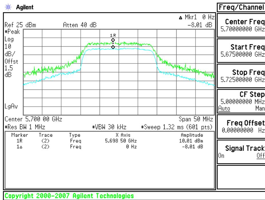
**Test mode: draft 802.11n Wide-40 MHz Channel mode / Chain 0+ Chain 1+ Chain 2:
