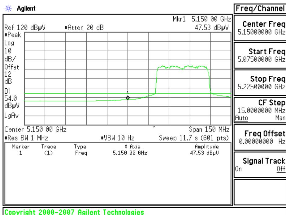
**Band Edges (draft 802.11n Standard-40 MHz Channel mode / 5310MHz)**
