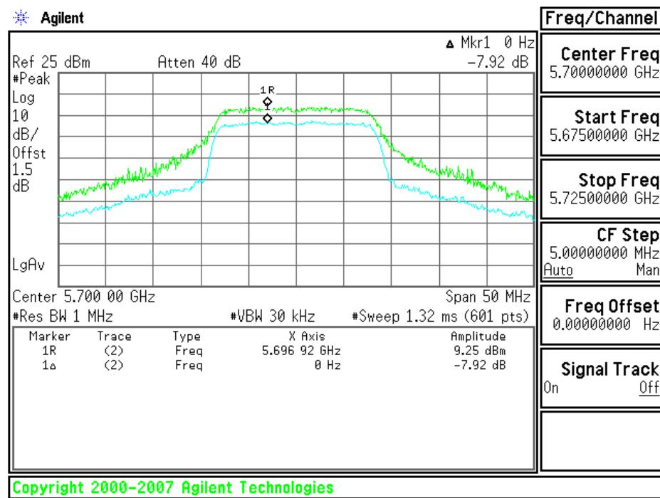
**Test mode: draft 802.11n Standard-20 MHz Channel mode / Chain 0:**
