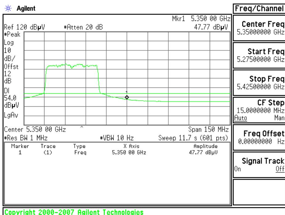
**Band Edges (draft 802.11n Standard-40 MHz Channel mode / 5510MHz)**
