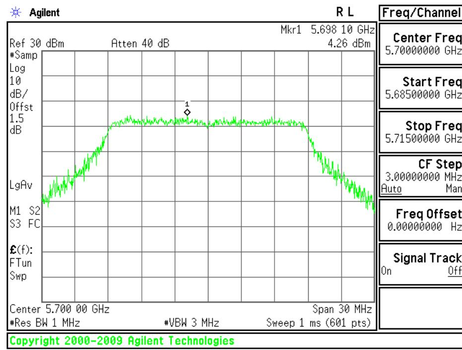
**Test mode: draft 802.11n Wide-40 MHz Channel mode / Chain 0:**
