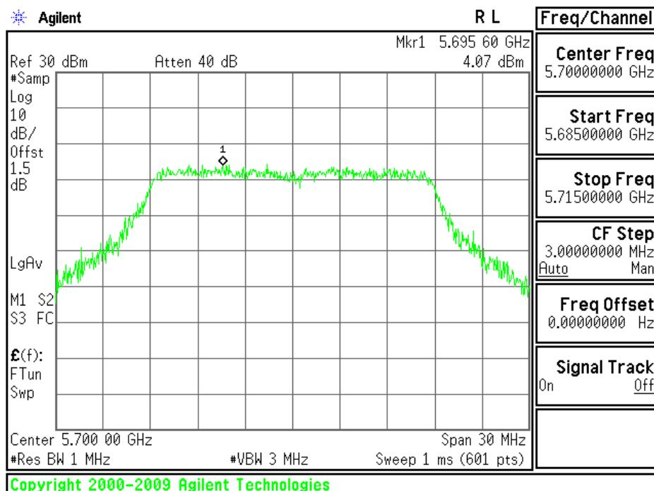
**Test mode: draft 802.11n Standard-20 MHz Channel mode / Chain 2:**
