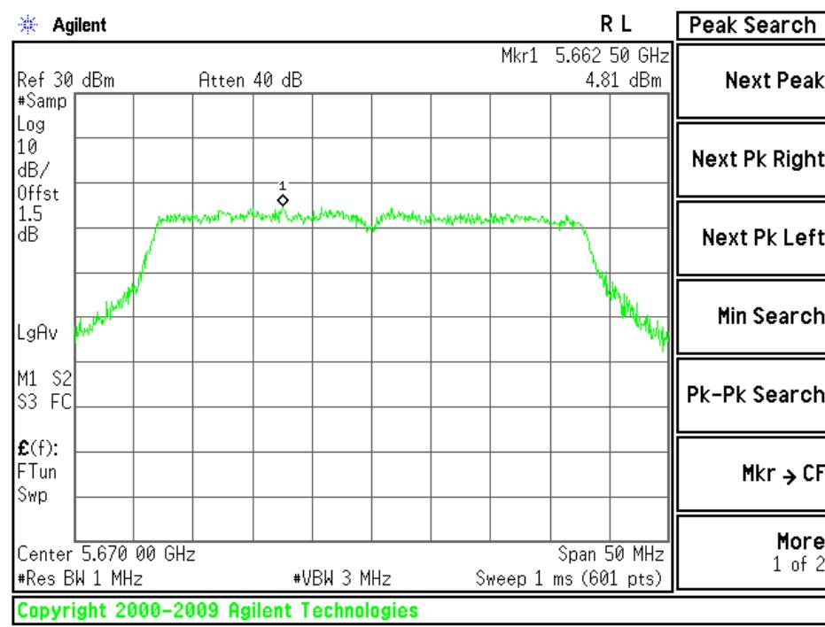
**Test mode: draft 802.11n Wide-40 MHz Channel mode / Chain 1:**
