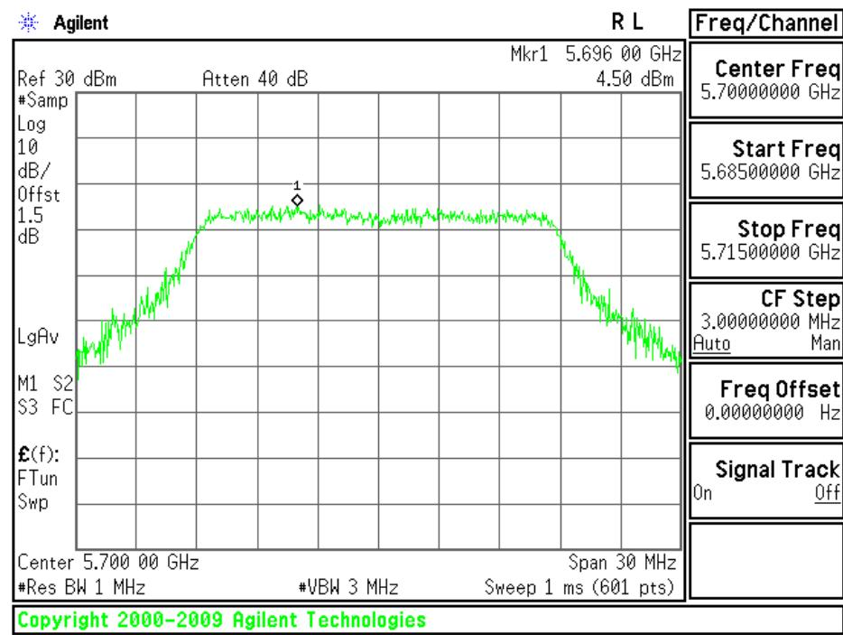
**Test mode: draft 802.11n Standard-20 MHz Channel mode / Chain 1:**
