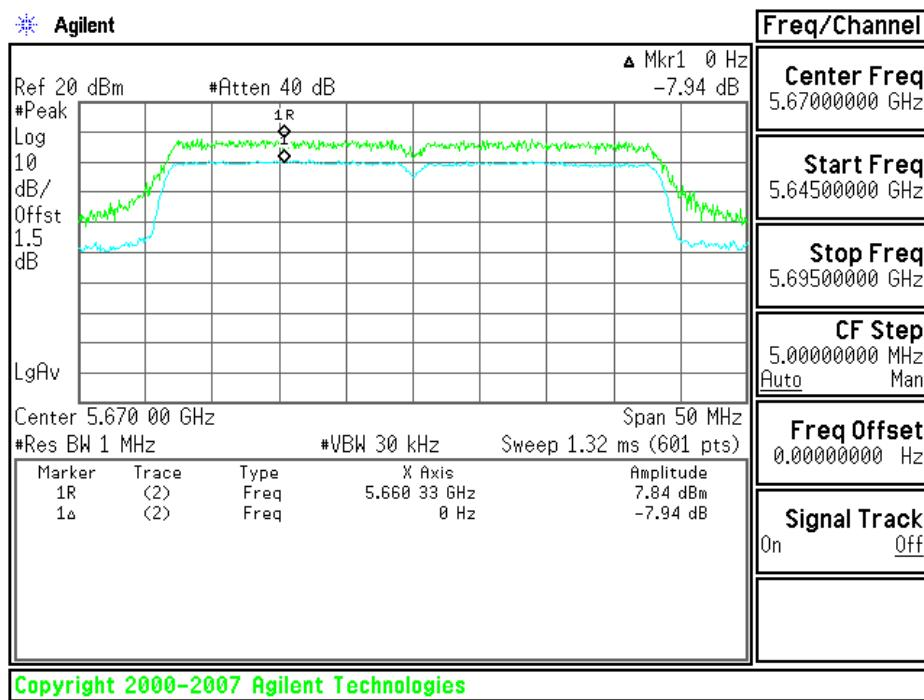
**Test mode: draft 802.11n Standard-20 MHz Channel mode / Chain 0+ Chain 1+ Chain 2:**
