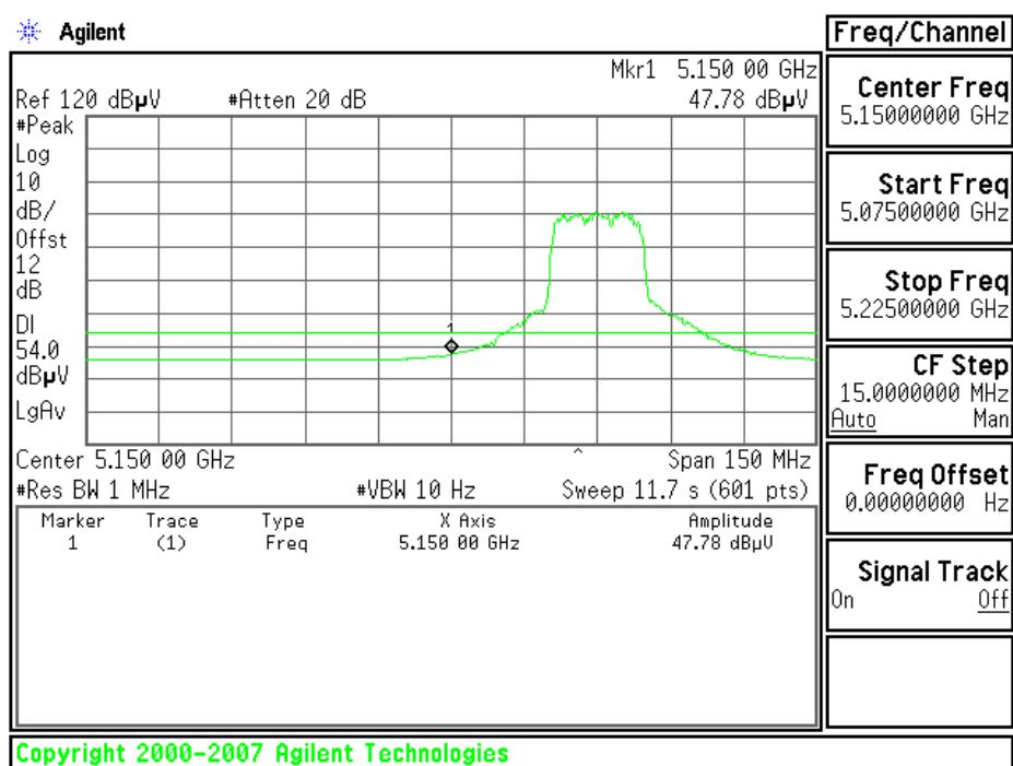
**Band Edges (draft 802.11n Standard-20 MHz Channel mode / 5320MHz)**
