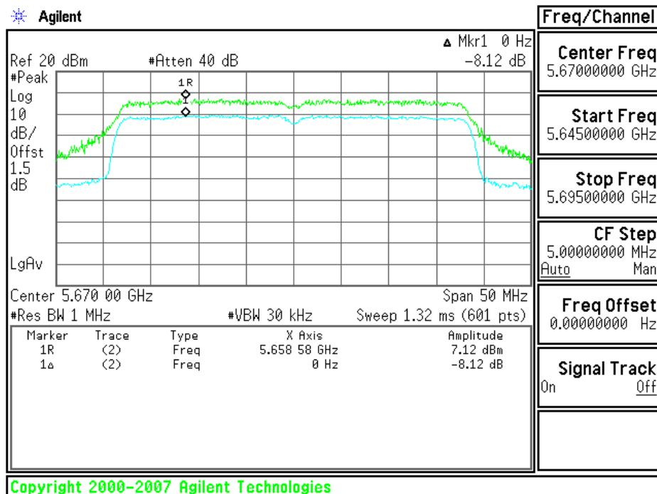
**Test mode: draft 802.11n Wide-40 MHz Channel mode / Chain 1:**
