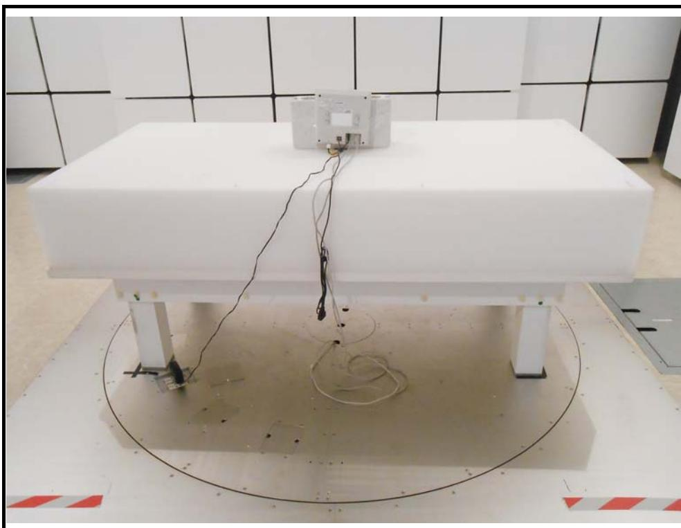
Radiated Emissions above 1 GHz Test
