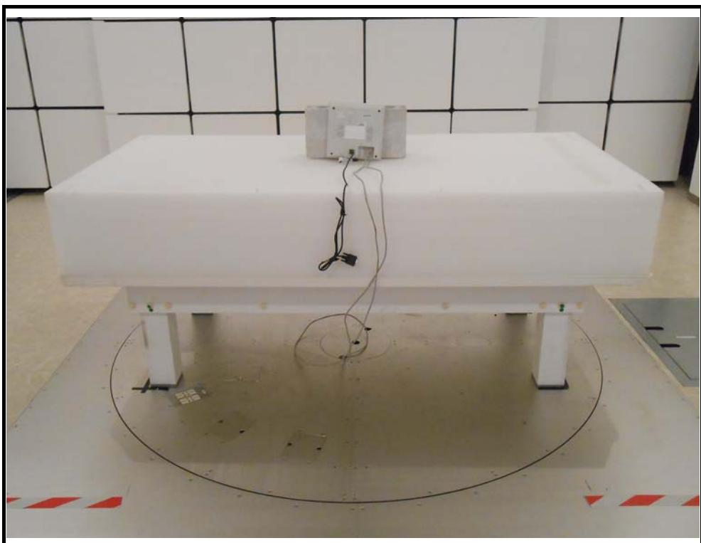
Radiated Emissions below 1 GHz Test
