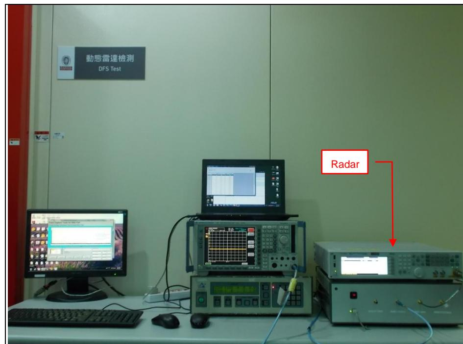
Set UUT as Master mode (Radar injected into Master) – Radio 2
