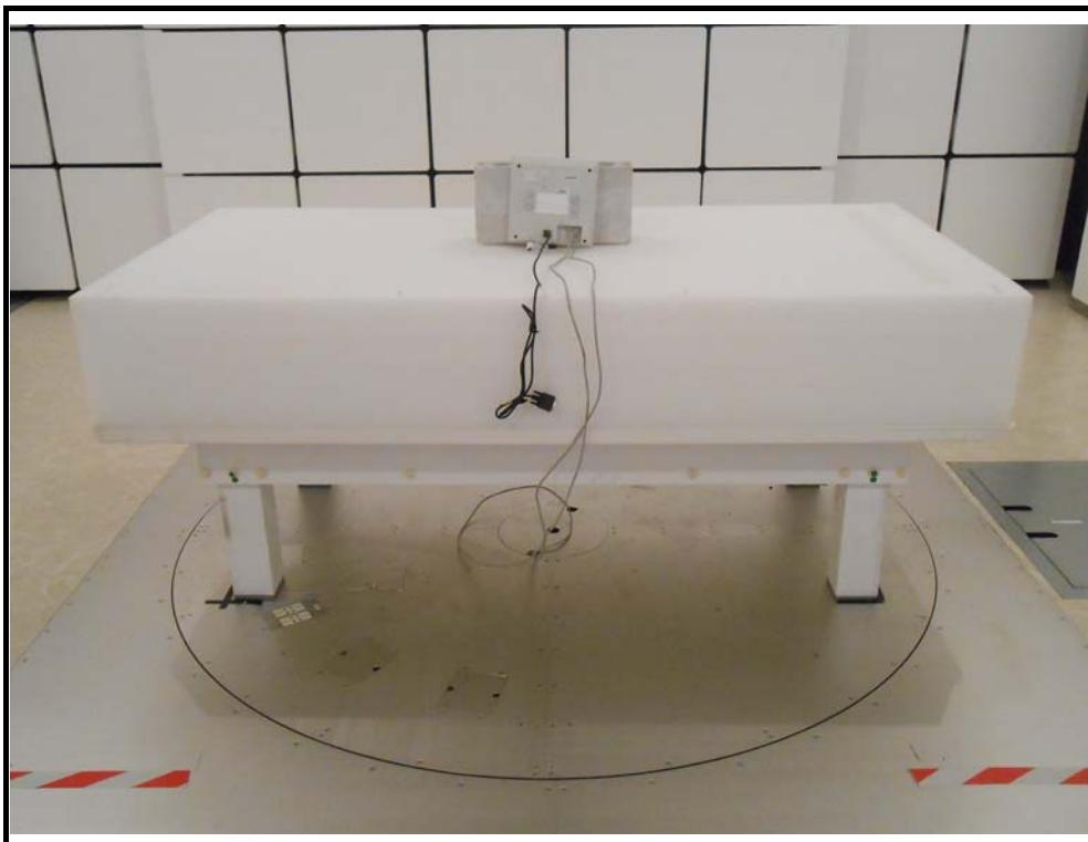
Radiated Emissions below 1 GHz Test
