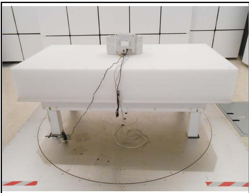
Radiated Emissions above 1 GHz Test
