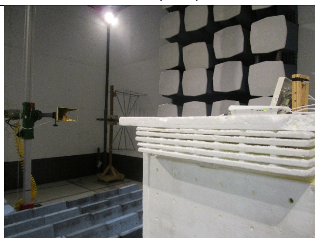
Radiated Emissions (>1GHz) – Rear View
