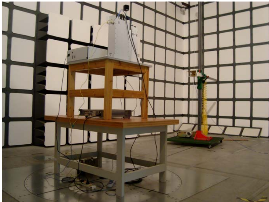
Above 1 GHz: Spurious Radiated Emissions - Rear View (Downlink mode)
