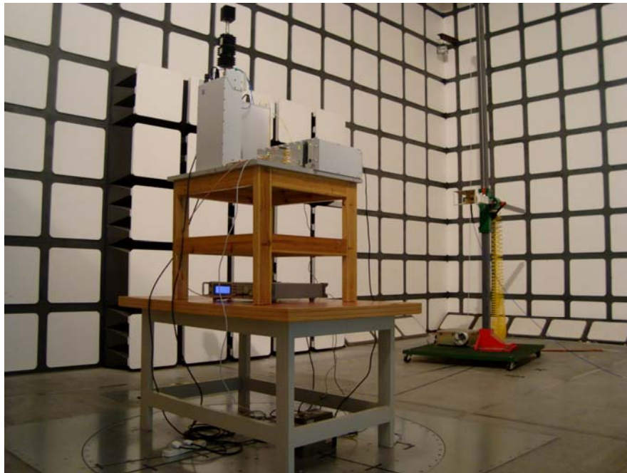
Above 1 GHz: Spurious Radiated Emissions - Rear View (Downlink mode)
