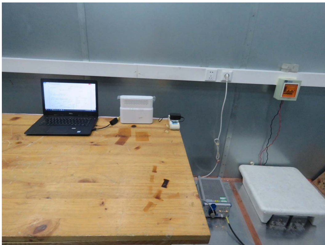
Picture 2 Conducted Emission Test Setup
