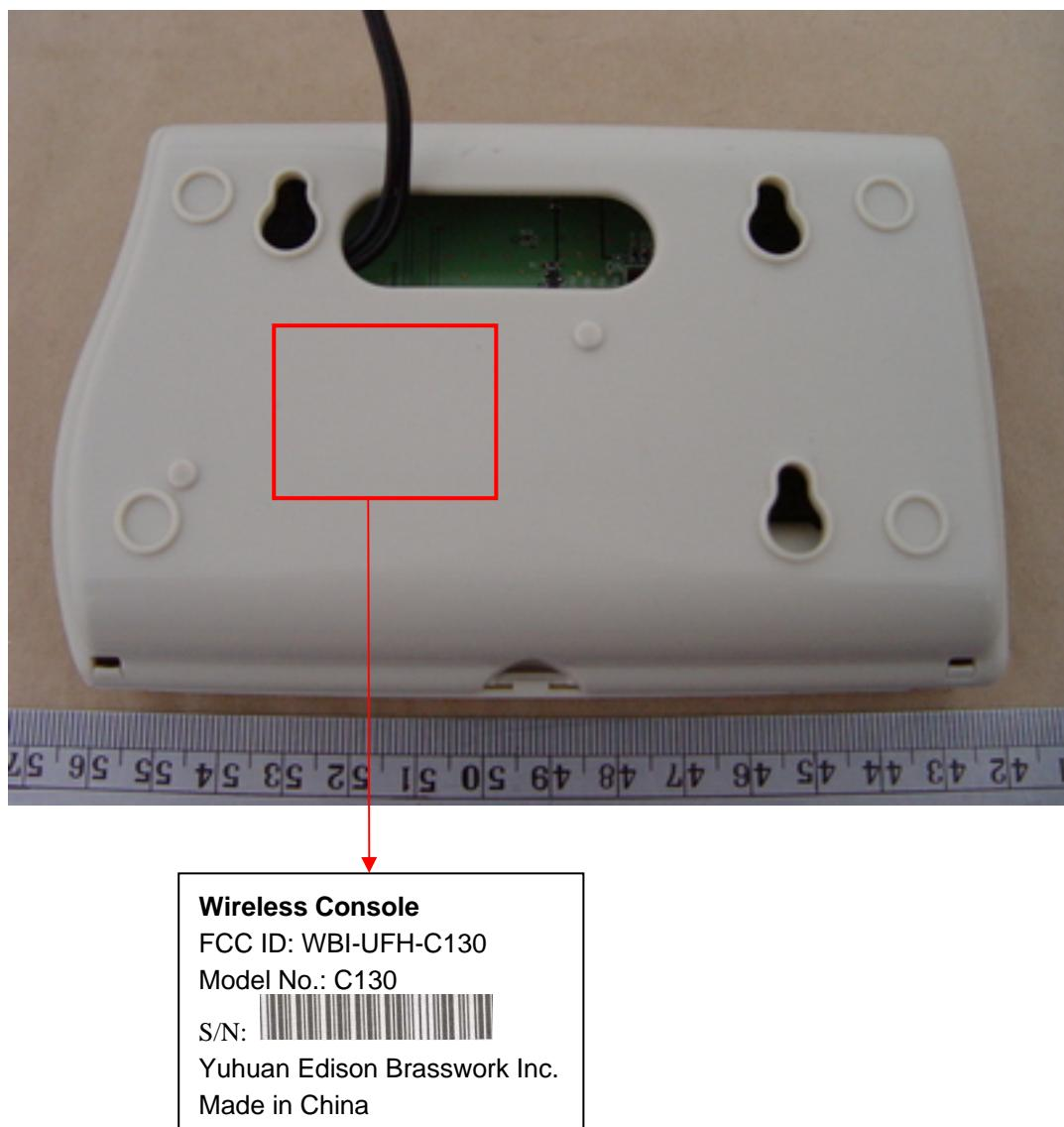
The label size is **40 mm X 30 mm** and because of the size of this device is too small to be placed the other required statement, the following will be placed in the user's manual:
