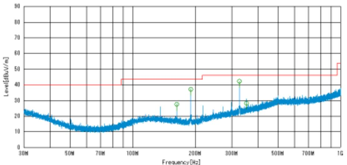
Antenna polarization: **Vertical** Maximum configuration: EUT – Z-Plane
