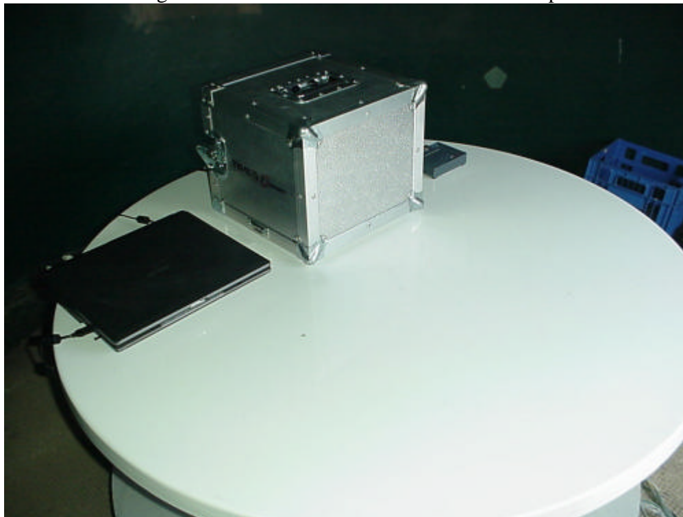
Registration reader radiated emissions test set up
