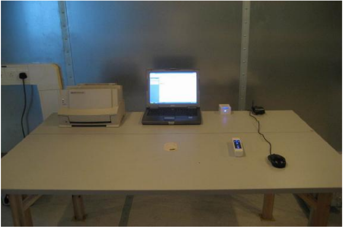
Measurement of Conducted Emission Test Set Up
