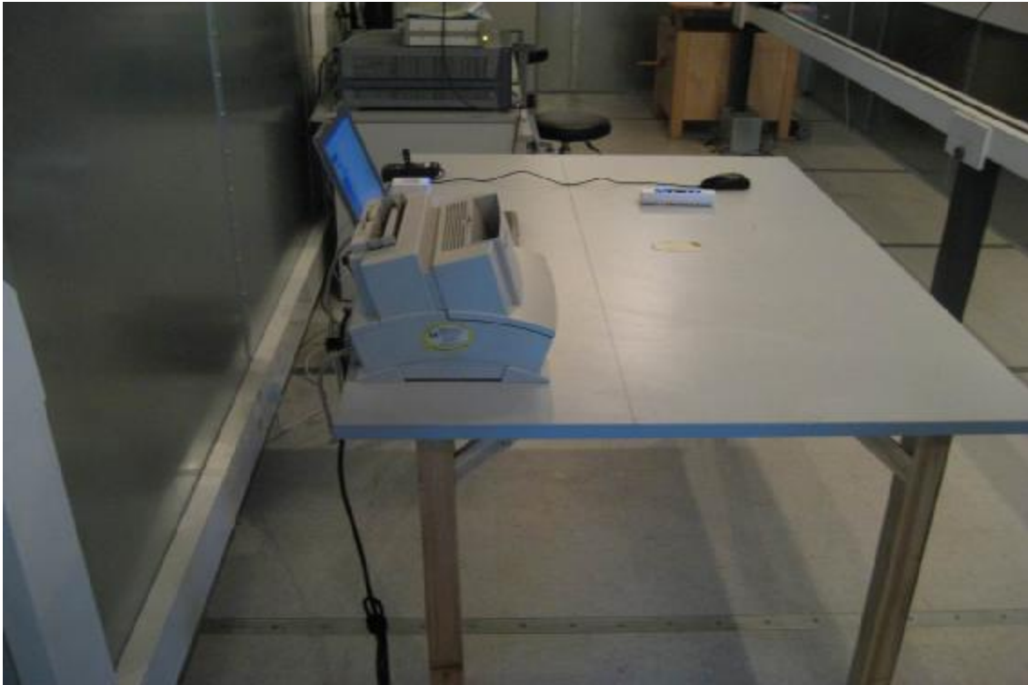
Measurement of Conducted Emission Test Set Up
